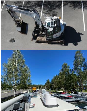
Figure 2. Smart Excavator of the University of Oulu (top), Omni directional antenna on the top of the machine (below).
