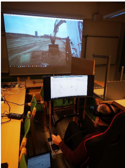
Figure 3. Remote control with VR glasses from the University of Oulu campus to the test site.
